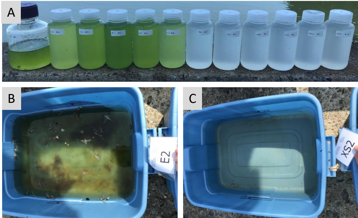
Figure 3. Photos of samples and mesocosms during algal bloom event. (A) Photo of samples collected from week 3 of experiment. Samples on the left were from uncovered mesocosms and samples on the right are from covered mesocosms. (B) Photo of an uncovered mesocosm and (C) a covered mesocosm during week 3.
